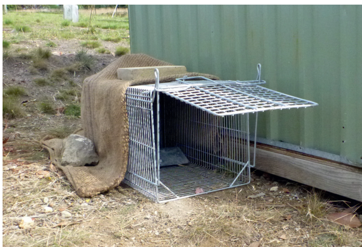
'Treadle-style' cage trap with back half covered with a hessian bag. Photo courtesy of Sue Robinson DPIPWE.
